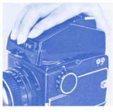
1. Place the rear part of the finder on the camera body while holding the front part of the finder slightly upward. Slide the rear part forward until it stops and gently lower the front part of the finder onto the camera body then firmly depress the finder downward. It will then lock into place.
